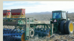
A Lawson aerator is a large, weighted drum pulled behind a tractor that crushes sagebrush and impacts the soil surface.
